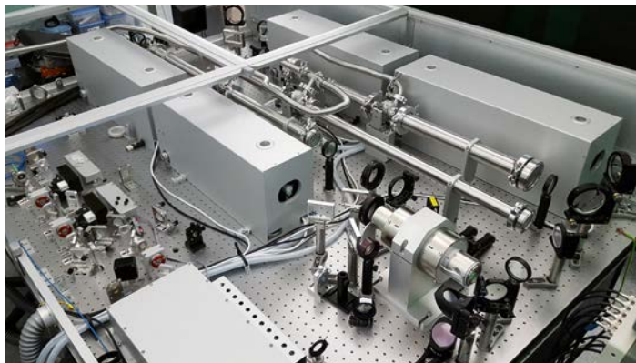
30 J Nd:glass system featuring arbitrary shaped temporal pulse shape
