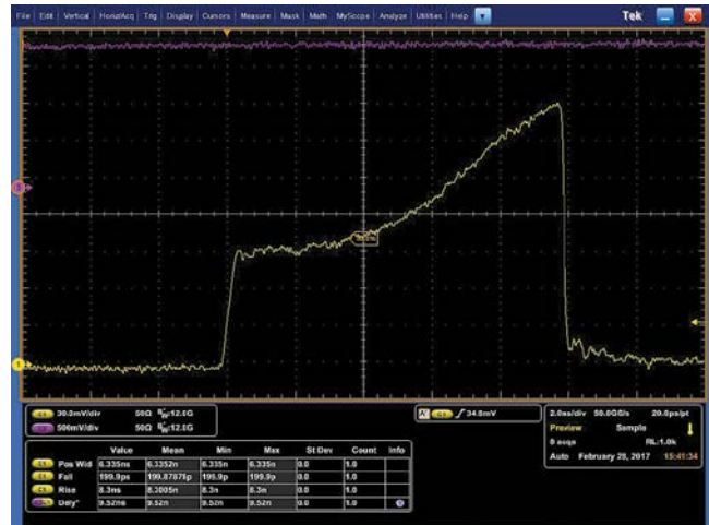
One example of the pulse wave form at the output @ 33 J (fundamental)
